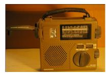
Hand crank portable radio. This model operates on batteries as well as AC power. Supports AM, FM and short wave frequencies and provides emergency lighting.
